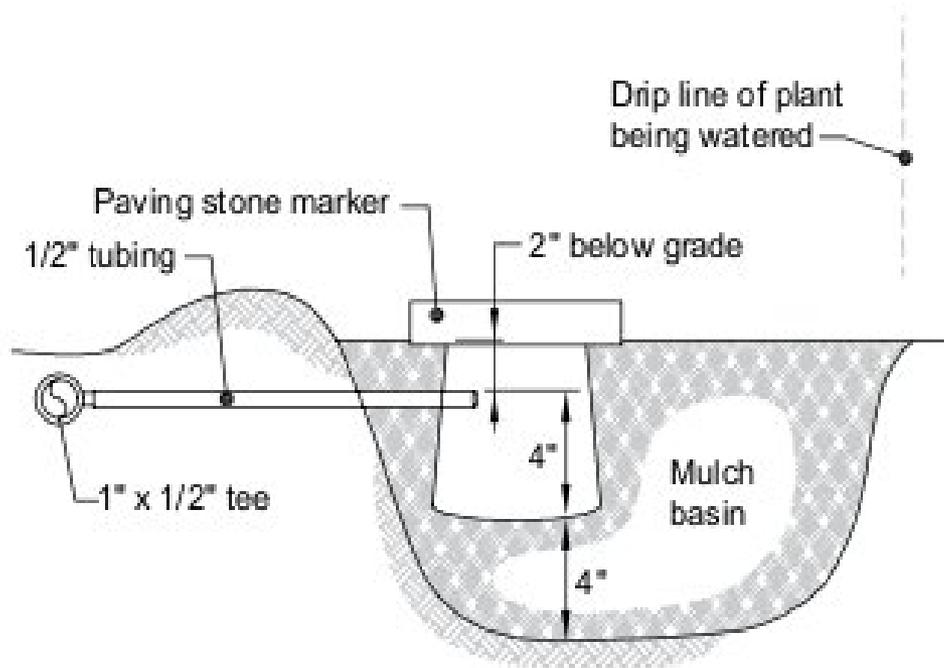
*Figure 4. Mulch shield placement.*
