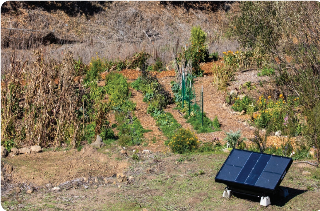
A solar-powered panel is capable of harvesting 4 to 5 liters of water per day from the air at the Hummingbird Farm Community Garden.
