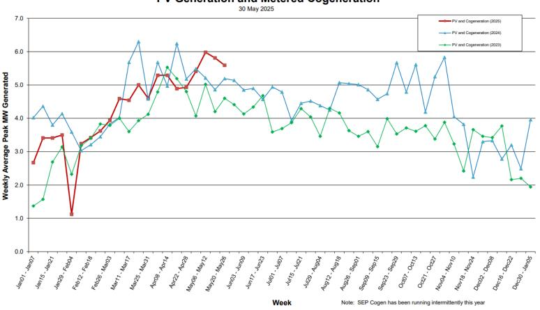
Solar Photovoltaic (PV) technology uses semiconductors to convert solar radiation into DC Electricity. Cogeneration is the process of capturing and using the by-products of electrical generation or wastewater treatment facilities. In the case of wastewater treatment facilities, cogeneration systems use the anaerobic digester gas to generate electricity. Rather than directly releasing these by-products back into the environment, they can be used to generate electricity for the facility.
