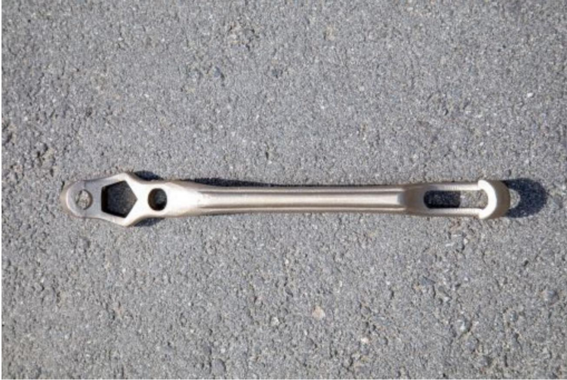
SFWD spanner wrench the ONLY permissible wrench for operation of hydrant valve spindle.
