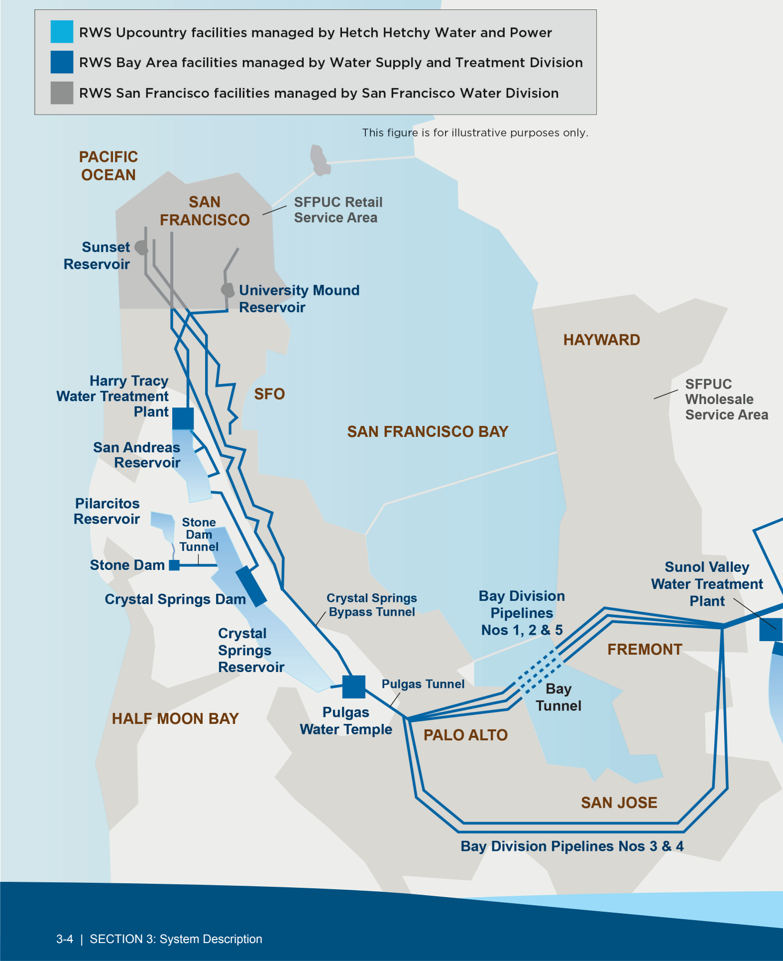
Figure 3-1. The Regional Water System and Main Facilities
