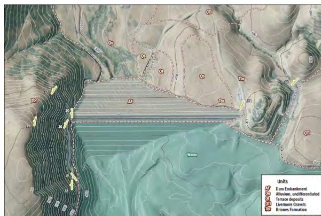
Turner Dam Site Geologic Characteristics; Left and Right Abutments Underlain by Briones Formation
