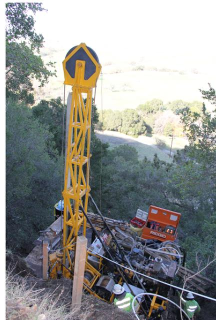
*Geotechnical Boring performed by Helicopter Access*
