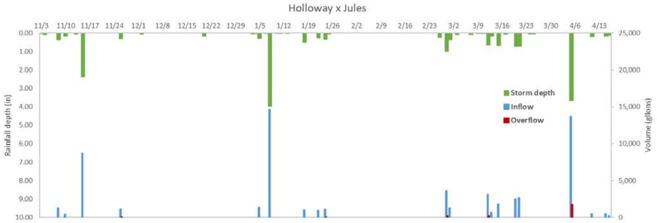
Figure 6: Hydrograph showing inflow and GI overflow of the 2017-2018 Monitoring Period at Holloway x Jules
