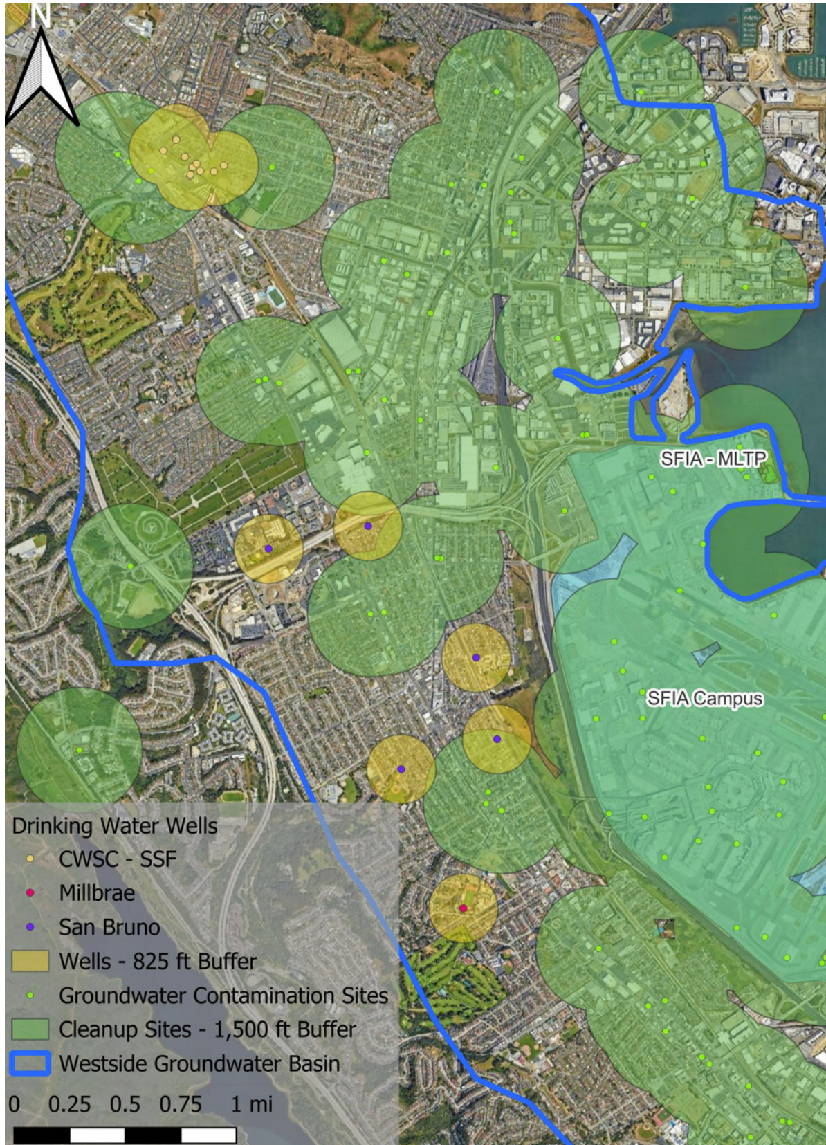
Figure 6.4 Groundwater Injection Well Siting Constraints
