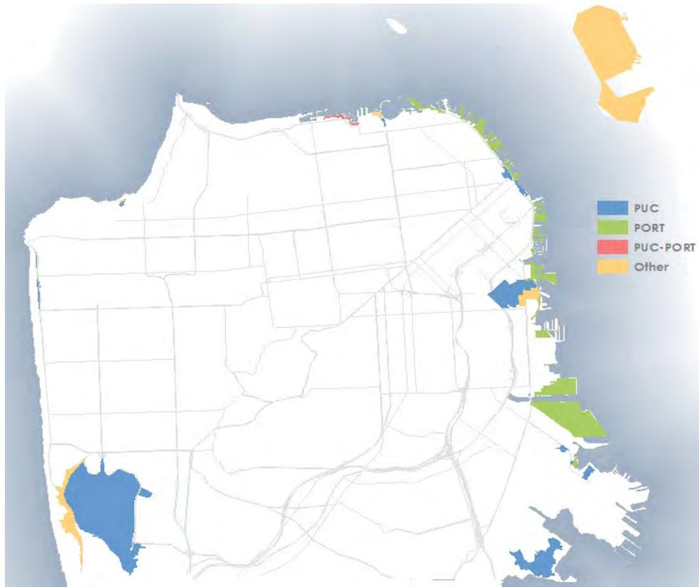
**Figure 1.** Separate sewer areas and jurisdictions. (Note: map is updated as-needed, for the most recent map go to [www.sfwater.org/smr](http://www.sfwater.org/smr))
