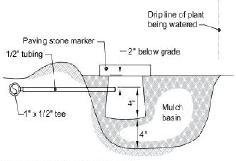
Figure 4. Mulch shield placement.
