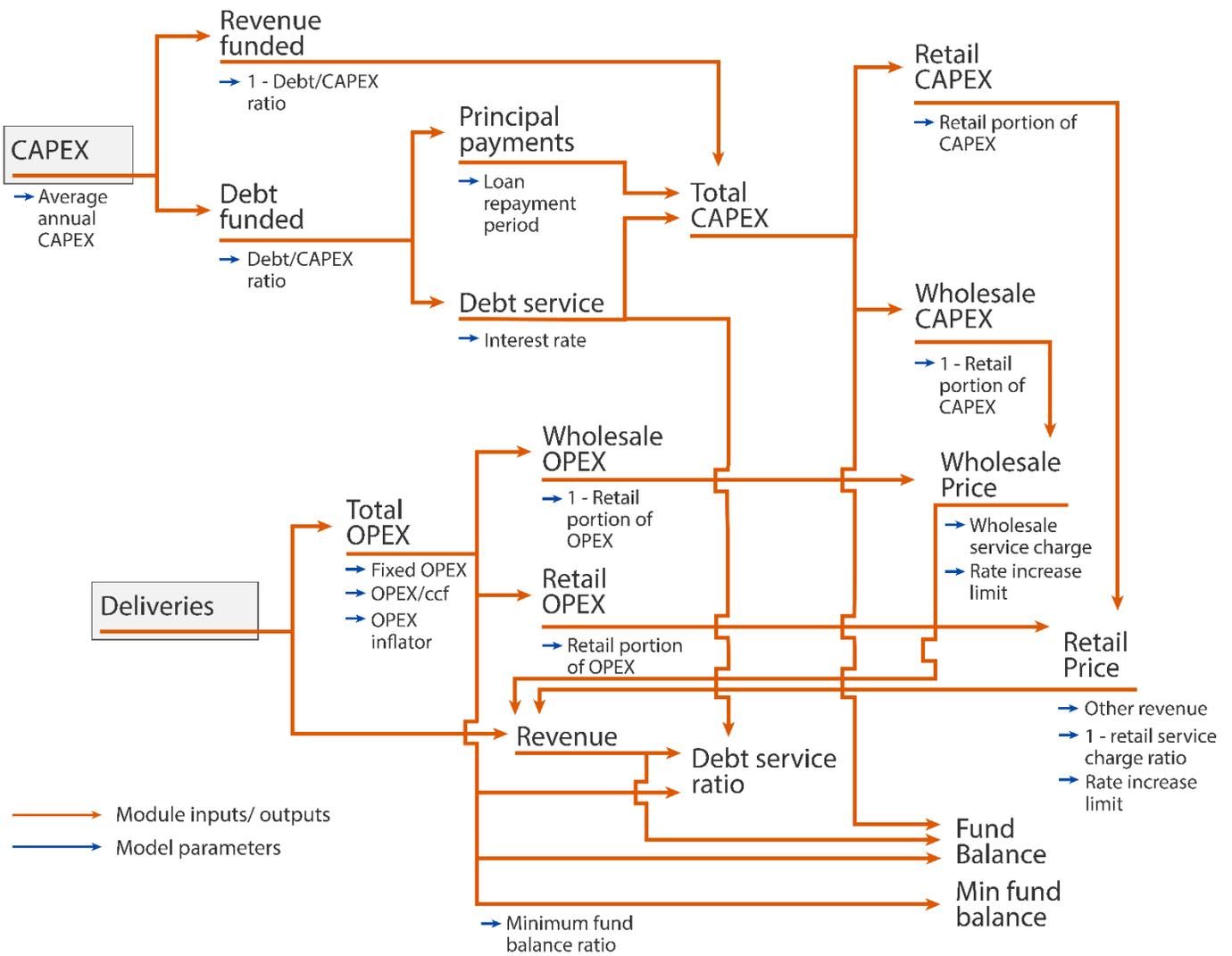
Figure 3: Schematic of finance module developed as part of LTVA. Orange arrows indicate model inputs/outputs and blue arrows indicate model parameters.
