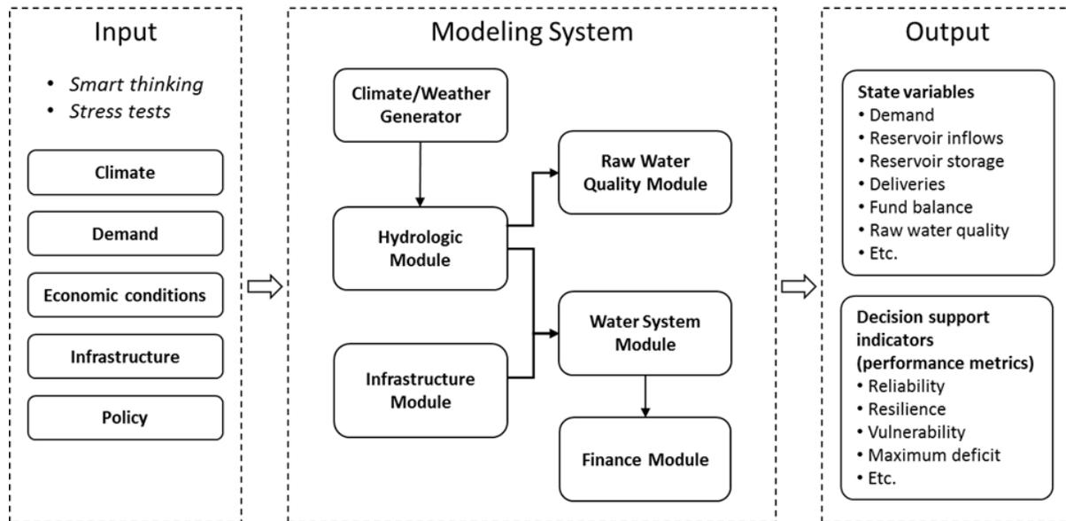
Figure 2: Conceptual diagram of the of LTVA modelling framework (including summary of inputs and outputs)
