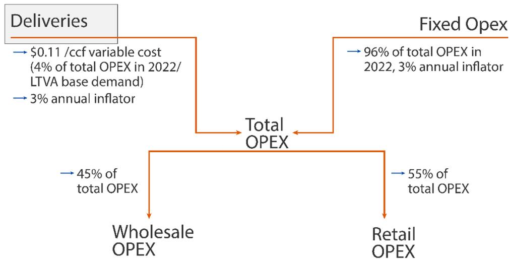
Figure 5: schematic of OPEX logic in LTVA Finance Module. Orange arrows indicate model inputs/outputs and blue arrows indicate model parameters.
