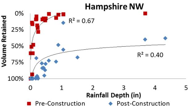
Figure 6. Estimated percentage of rainfall volume retained within each bioretention unit per storm event relative to the storm total rainfall depth based on modeling results.
