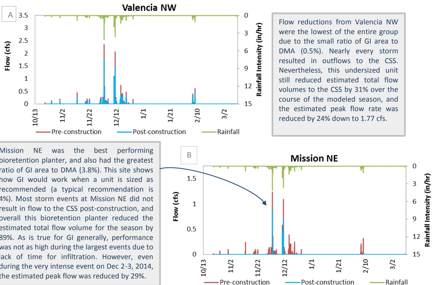
Figure 2. Modeled pre-construction versus post-construction flows and rainfall intensity at Cesar Chavez bioretention sites A) Valencia NW and B) Mission NE for the 2014-2015 rainy season.
