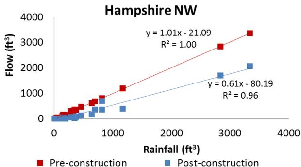
Figure 5. Rainfall and estimated flow volume for all individual storm events during Rainy Season 2014-15 at each bioretention unit based on model results.
