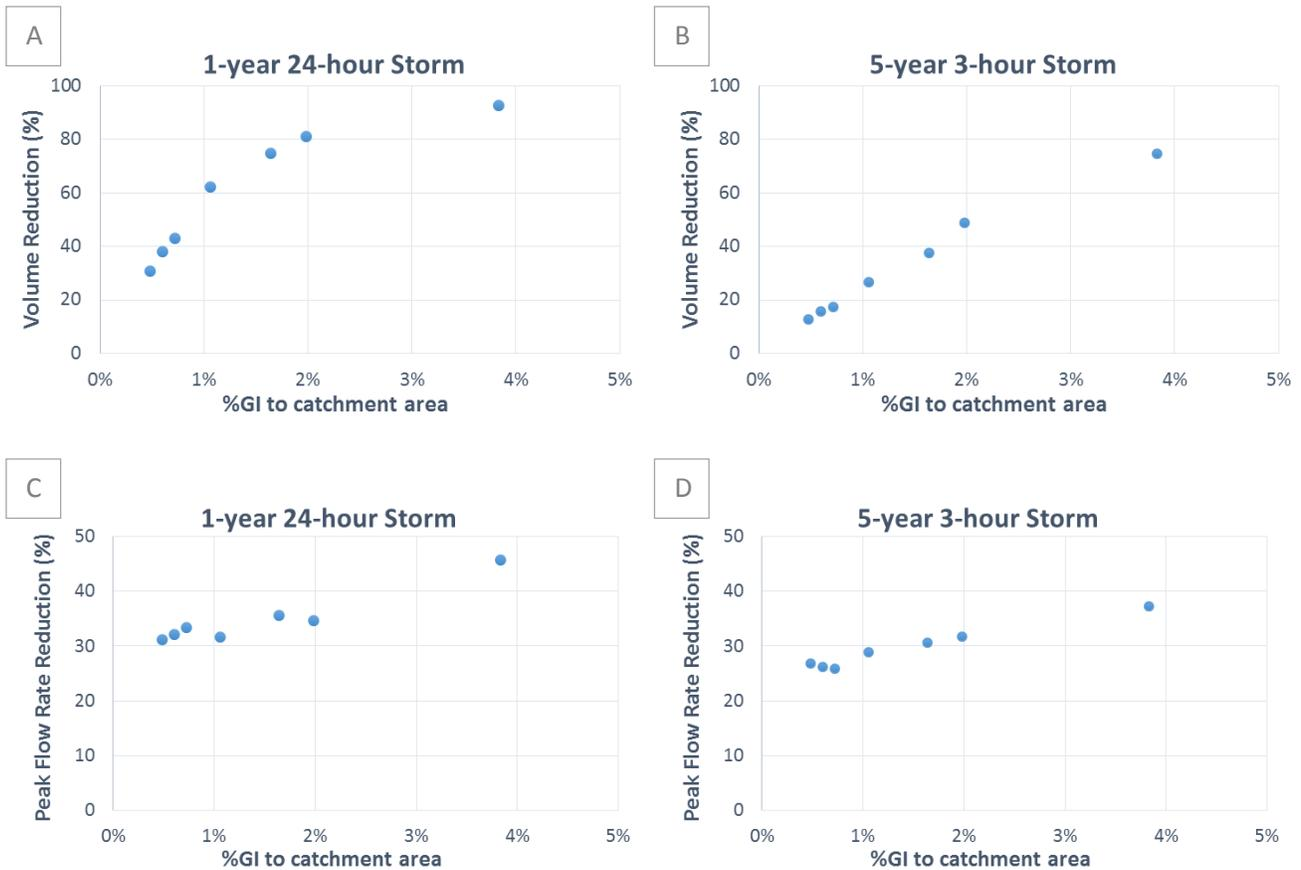
**Figure 3. Estimated flow volume reduction in relation to the ratio of GI area to DMA for the A) 1-year 24-hour storm, and B) 5-year 3-hour storm. Estimated peak flow rate reduction in relation to the ratio of GI area to DMA for the C) 1-year 24-hour storm, and D) 5-year 3-hour storm.**
