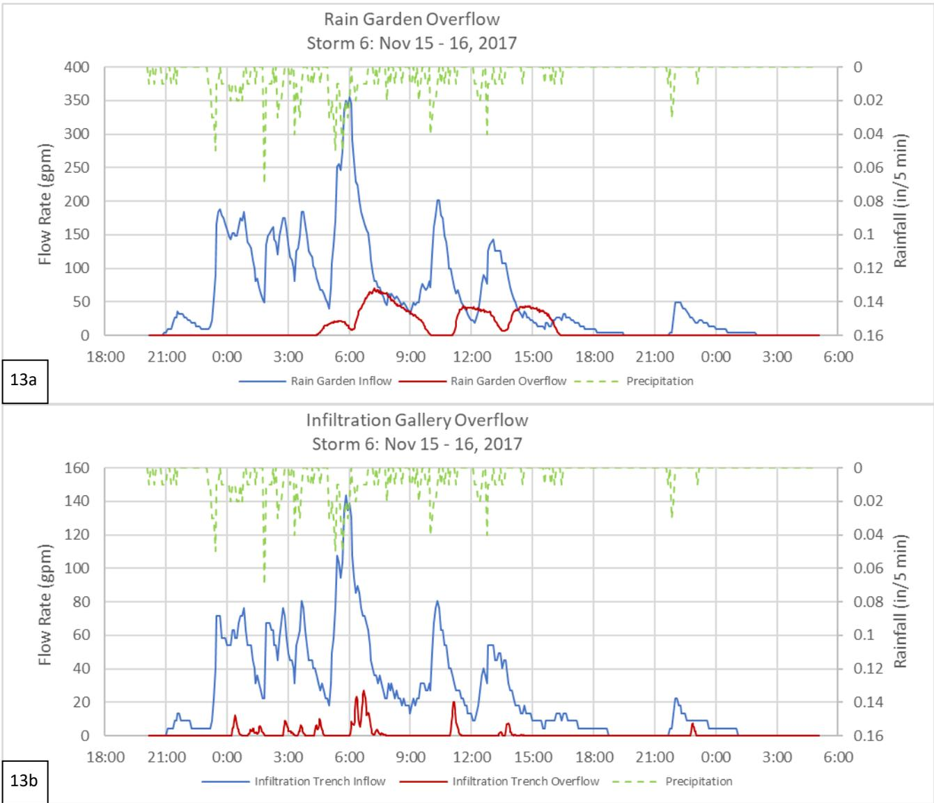
Figure 8a and 13b: Hydrographs for Storm 6 at the MVGG rain gardens and infiltration gallery
