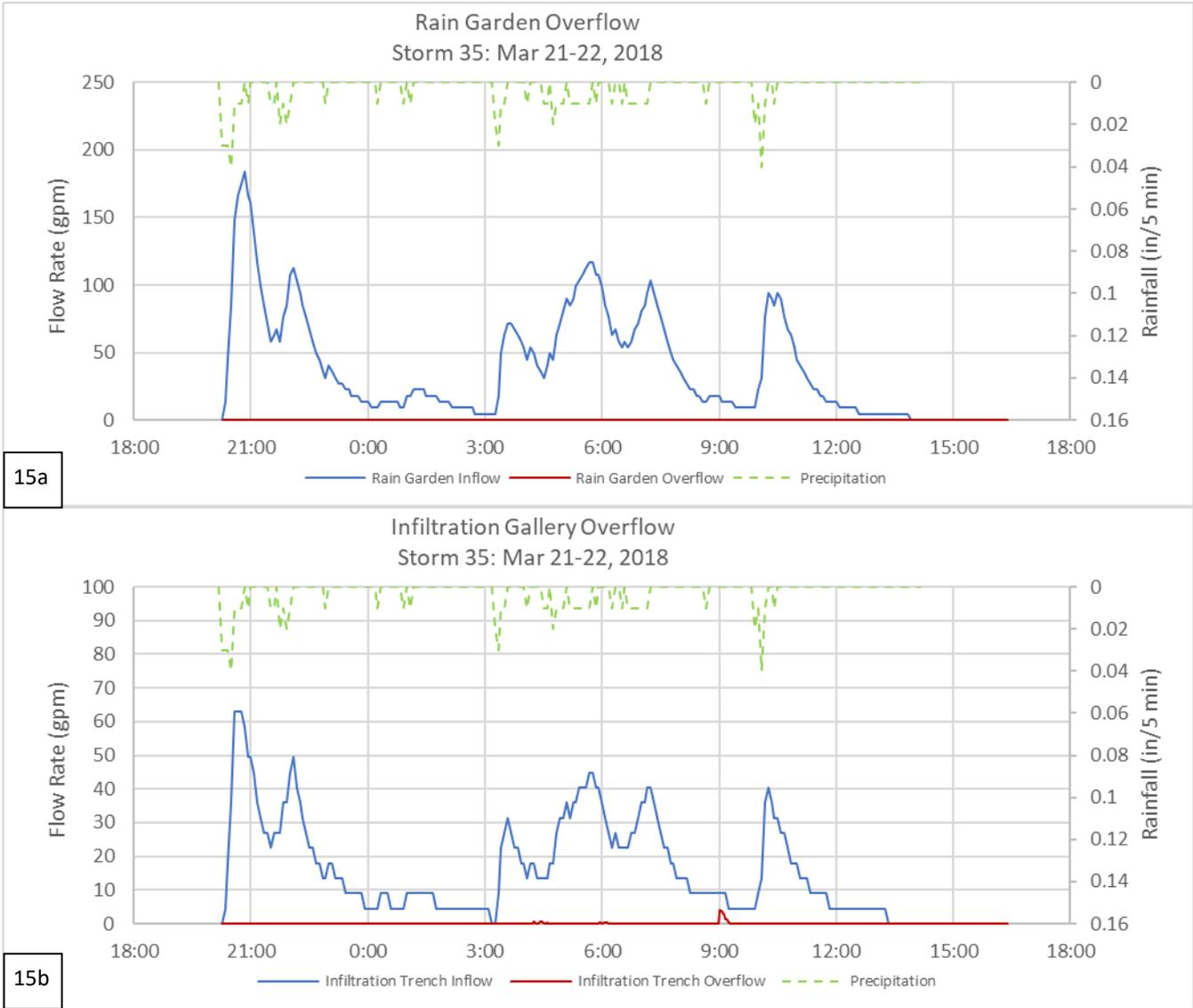
Figure 10a and 15b: Hydrograph for Storm 35 at the MVGG rain gardens and infiltration gallery
