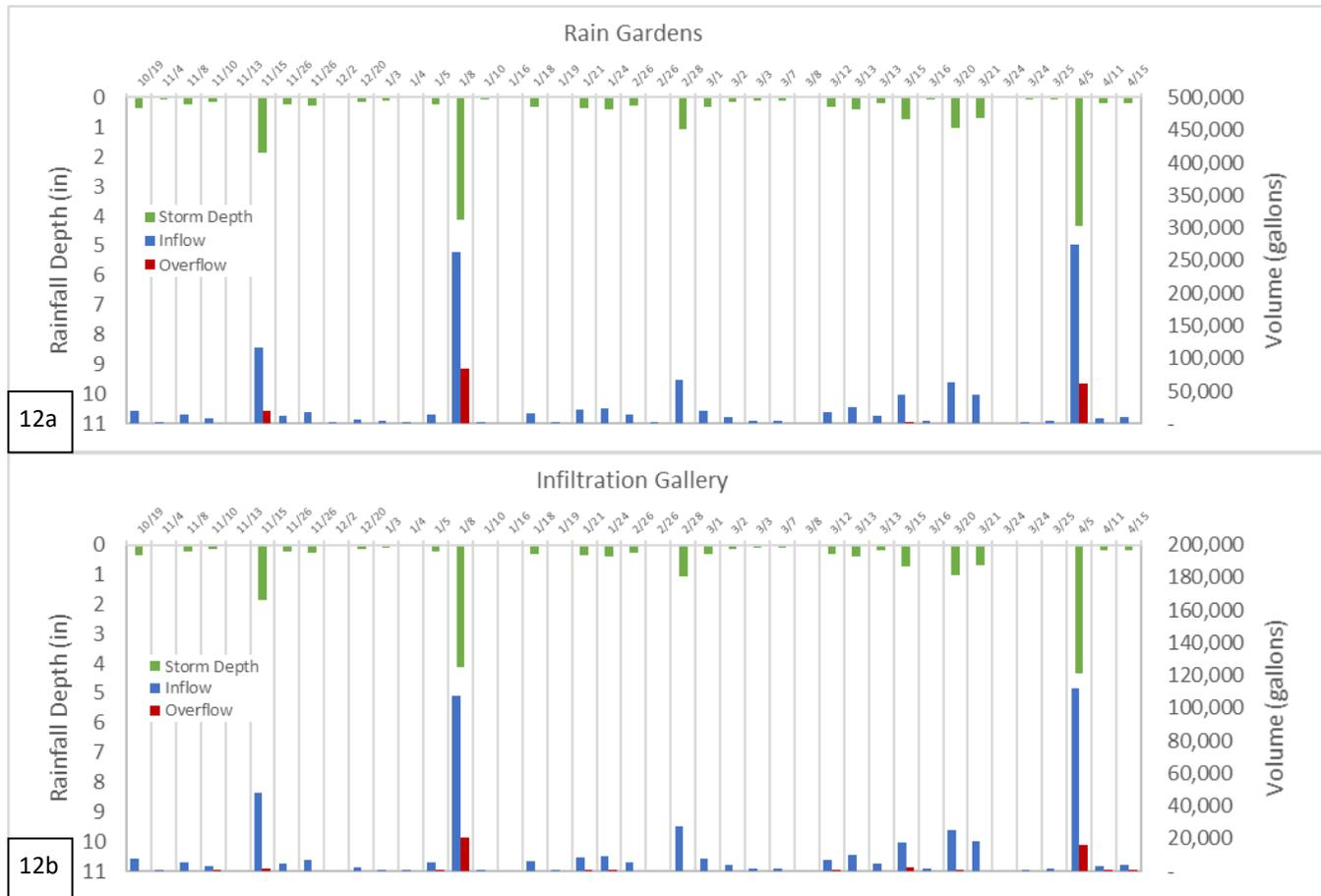
Figure 7a and 12b: Hydrographs showing inflow and outflow at the MVGG rain gardens and infiltration gallery
