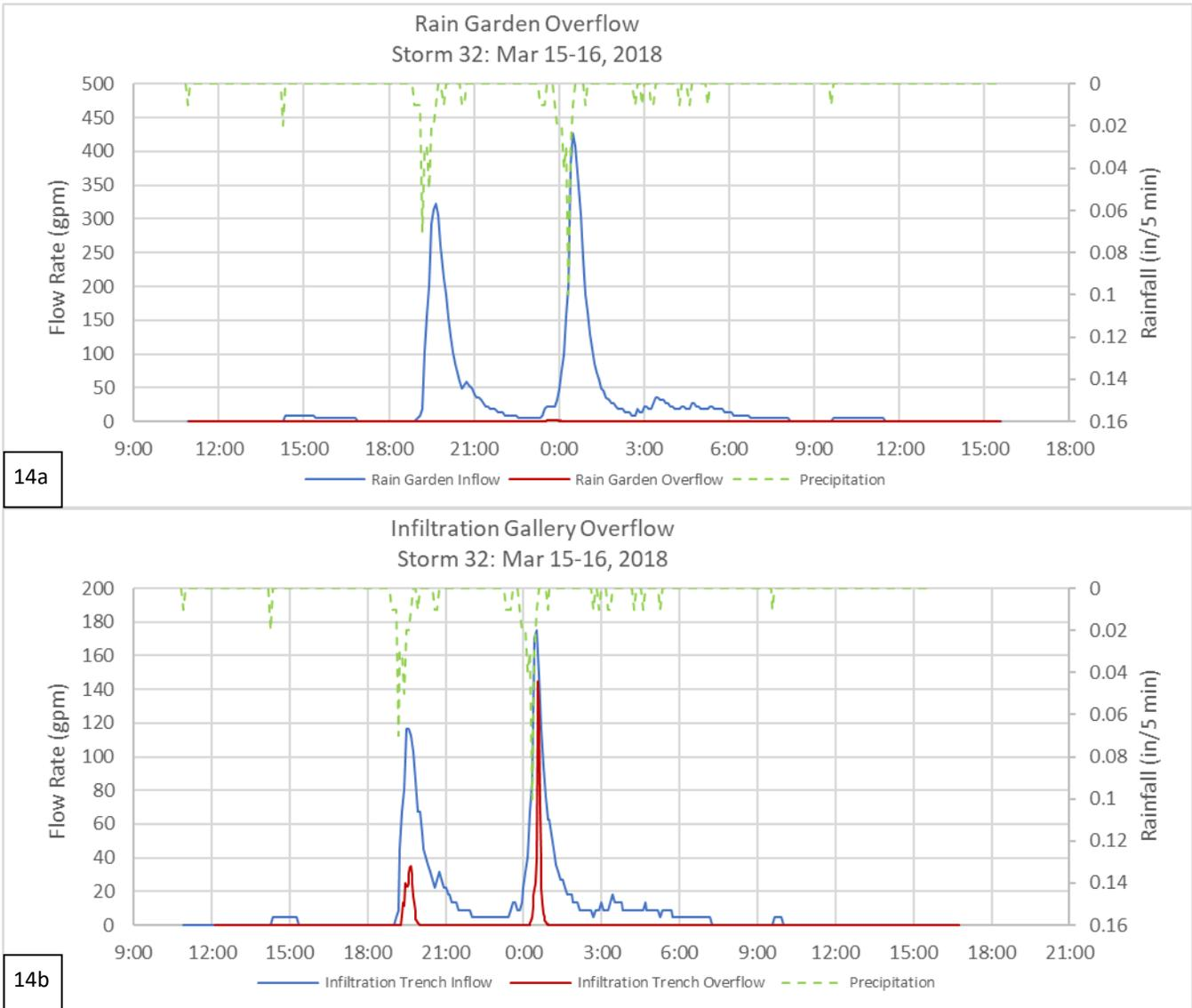
Figure 9a and 14b: Hydrographs for Storm 32 at the MVGG rain gardens and infiltration gallery
